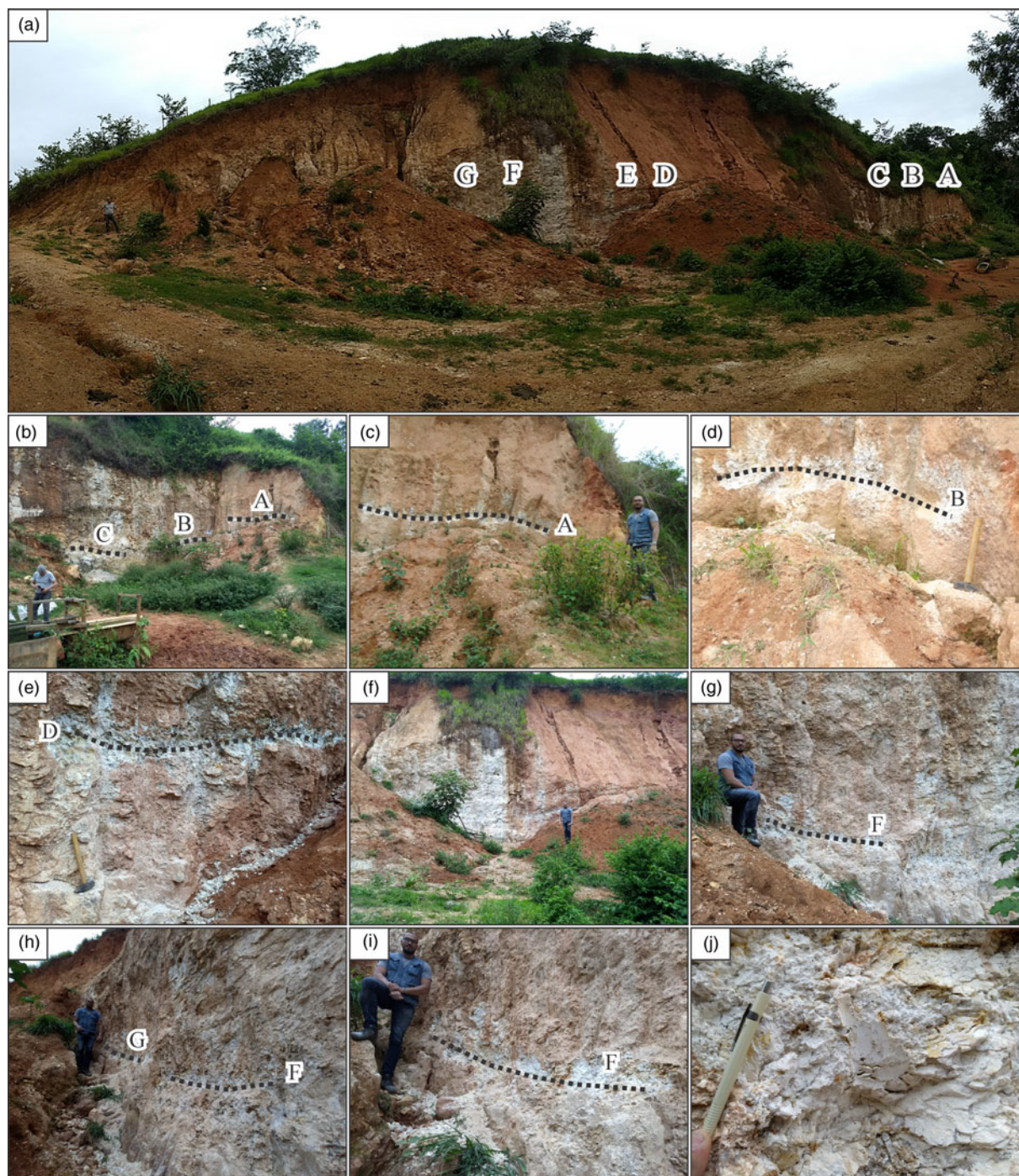
Fig. 2. Channel sampling sites located along the face of the pegmatite. (a) Overview of the outcrop of Exposição pegmatite. (b) Overview of the right part of the outcrop with the location of horizontal channels, where the samples A, B and C were collected. (c) The right part of the outcrop, where sample A was collected in a 4 m-long channel. (d) Sampling location of sample B in a channel 4.2 m long. (e) The left part of the outcrop, where sample D was collected in a horizontal channel 2 m long. (f) Detail of the left part of the outcrop. (g) Sampling location of sample F on the left part of the outcrop. (h & i) Close views of the segments where samples G and F were collected in horizontal 2.0 and 2.5 m channels, respectively. (j) Details of the kaolin occurrence in the pegmatite.
