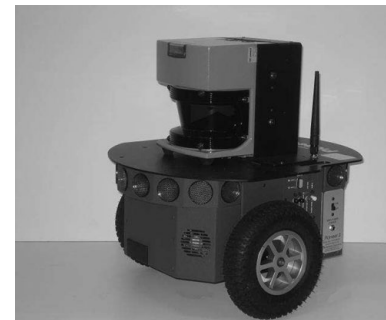
Fig. 17. Pioneer 3-DX robot which is equipped with Laser and Sonar range finders.
