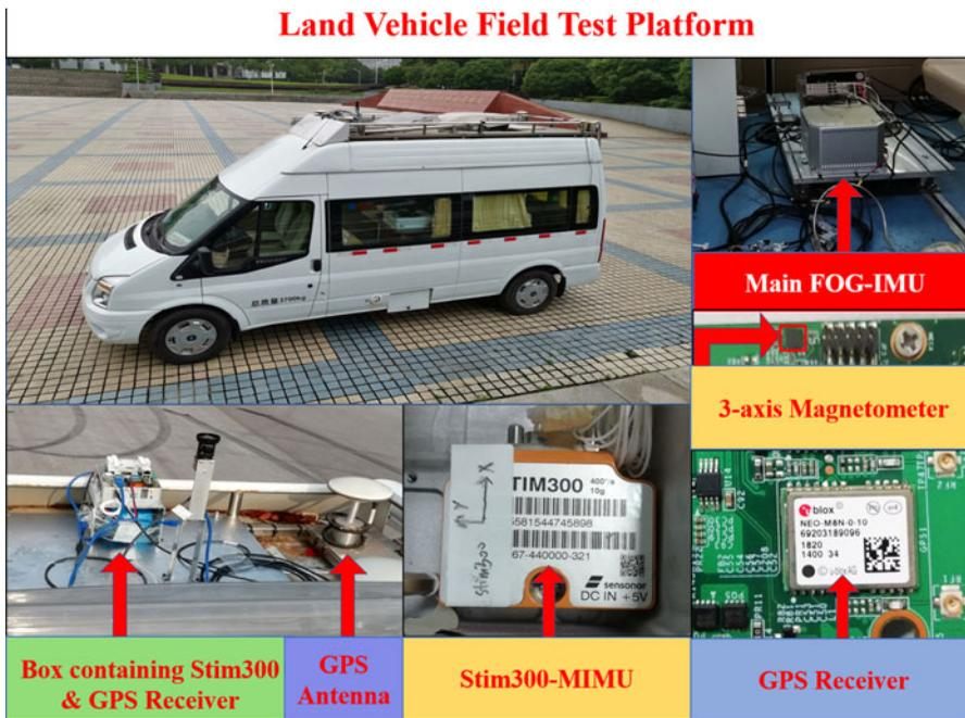
Figure 1. Sensor configurations of the land vehicle field test.
