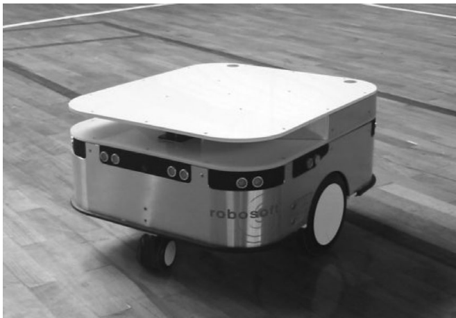
Fig. 8. RobuLAB 10 wheeled mobile platform.
