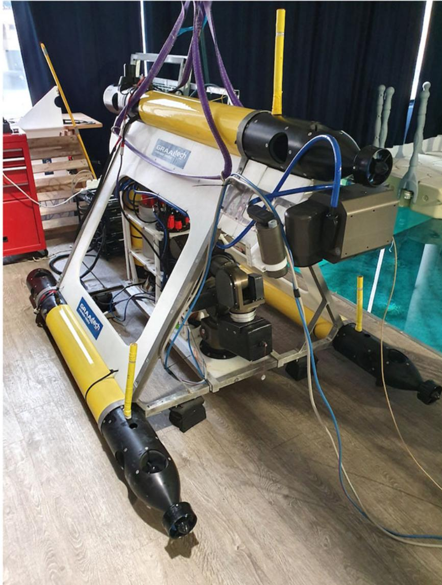
Fig. 1. The H2020 ROBUST project UVMS (Underwater Vehicle Manipulator System) platform.
