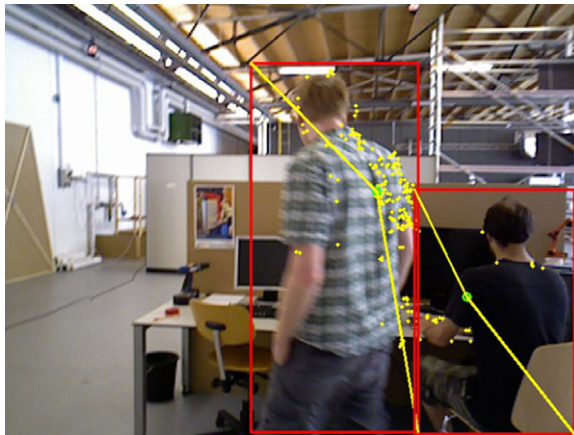
Figure 10. Boxes tracked by the box tracking method. The red boxes are the bounding boxes; the yellow dots are the seed points; the green dot is the mean point; and the yellow lines indicates the vectors used to obtain the two corners of a bounding box.
