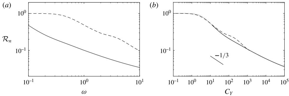
FIGURE 11. Shear reconfiguration number in the large-amplitude regime for  $\lambda = 12.7$ , against (a) the frequency ratio  $\omega$ , (b) the Cauchy number  $C_Y$ , for  $\alpha = 10^0$  (---),  $\alpha = 10^1$  (—). Static solution obtained with (5.6) (⋯⋯⋯, on (b) only).
