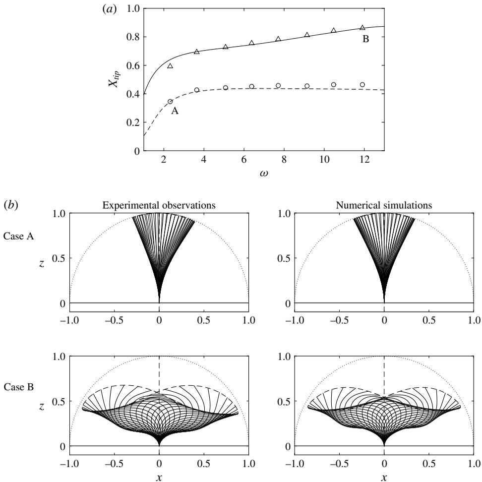
FIGURE 4. Comparison between experimental observations and numerical simulations. (a) Amplitude of the deflection at the tip against the frequency ratio, for  $\alpha = 0.27$  (numerical —, experimental  $\circ$ ),  $\alpha = 0.65$  (numerical —, experimental  $\triangle$ ). (b) Deformed shape found experimentally (left) and numerically (right), in case A (top,  $\alpha = 0.27$ ,  $\omega = 2.3$ ) and case B (bottom,  $\alpha = 0.65$ ,  $\omega = 12.0$ ).
