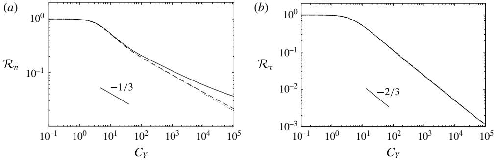
FIGURE 14. Variations of the static reconfiguration numbers obtained with (5.6) ((a) shear, (b) tensile) as a function of the Cauchy number  $C_Y$ , for  $\lambda = 12.7$  (—),  $\lambda = 127$  (---),  $\lambda = 1270$  (·····).
