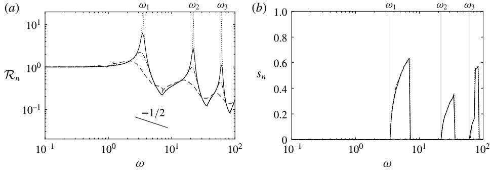
FIGURE 9. Shear reconfiguration number (a) and location of maximum shear stress along the span (b), in the modal regime, against the frequency ratio, for  $K_C = 10^{-2}$  (—),  $K_C = 10^{-1}$  (— · —),  $K_C = 10^0$  (---) and analytical solution for  $K_C \rightarrow 0$  (·····).
