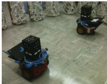
Fig. 12. Two Pioneer P3-DX robots equipped with cameras and targets. Robot 1 is shown on the left, while robot 2 is on the right.
