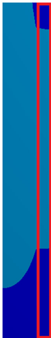
Fig. 8. 2D-axisymmetric representation of the solidification line for a filling time of 25 minutes. Red zone represents edges of the steel cell.
