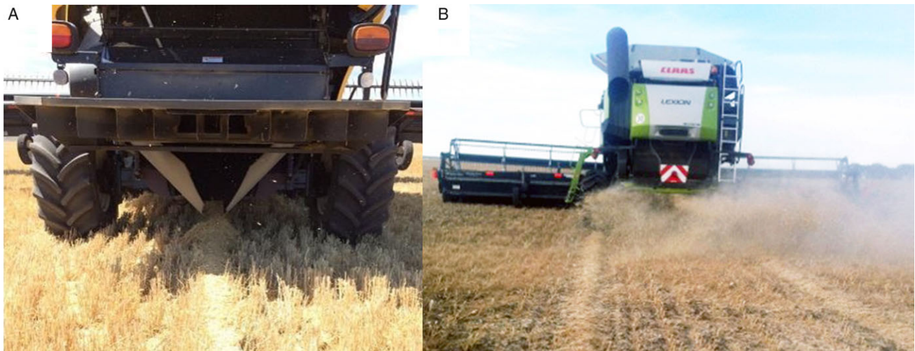
Figure 1. Harvest weed seed control systems that concentrate the weed-containing chaff fractions into narrow rows (20 cm) during harvest. (A) Chaff lining and (B) chaff tramlining.
