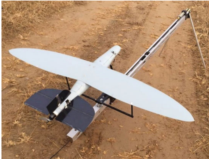
Figure 1. (Colour online) The bio-inspired wing SUAV prototype.
