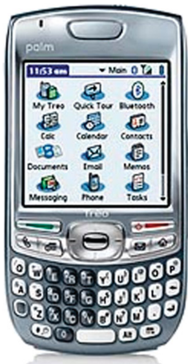
Fig. 2. The Treo 680 smartphone [111.8 mm (l) × 58.4 mm (w) × 20.3 mm (d); 157 g] runs on the Treo OS 5.4.9 platform. It has an Intel PXA270 312 MHz processor, a 320 × 320-pixel TFT touch screen, 64 MB of nonvolatile flash memory (with more storage capacity available via external expansion card), GSM/GPRS/EDGE class 10 radio quad band, a 1.3-megapixel VGA camera with 2× digital zoom and video capture, removable rechargeable battery, and built-in infrared technology.
