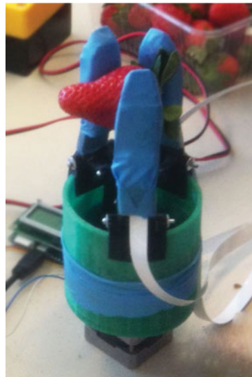
Fig. 5. Functional experimental prototype of the gripper created on a 3D printer, grasping a fresh strawberry.
