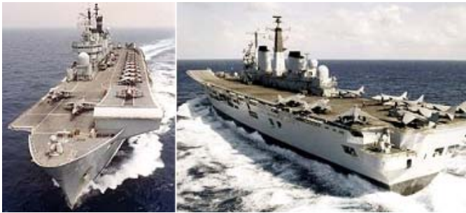
Figure 4. HMS Illustrious with retrofitted 12° ramp.
