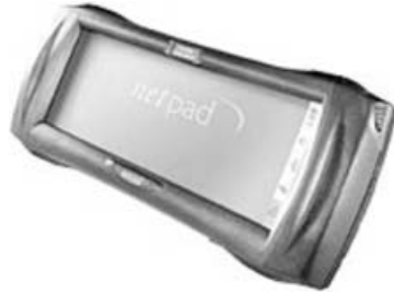
Figure 2. The Psion Netpad, a portable unit for use with the on-board Pilot Port.
