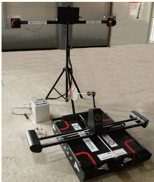
Figure 1. The whole badminton robot system. It contains the infrared-based binocular vision subsystem and the robot subsystem which consists of the chassis motion subsystem of four Mecanum wheels, the two-dimensional platform servo subsystem and the ball striking system.
