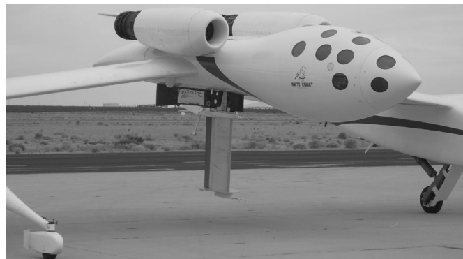
Figure 27. FlexSys MACW installed on White Knight for flight tests (59) .
