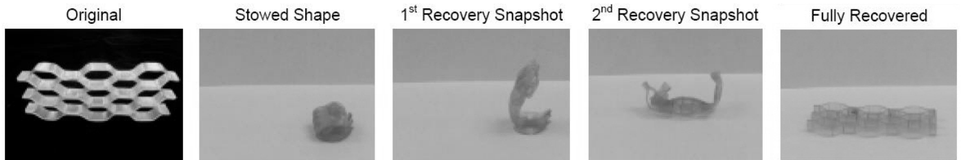
Figure 17. Veriflex ® honeycomb structure self-recovering under an IR heat lamp (99) .
