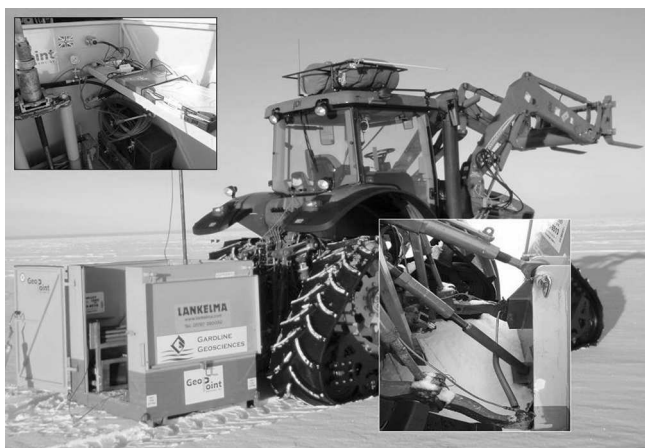
Fig. 1. UK11 configured and fitted for CPT. Insets show rigid-link installed and data-collection equipment.
