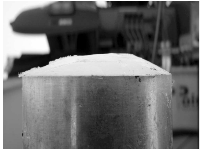
Fig. 11. Low-angle conical plug routinely observed on a flat plate post-test. The flat plate has a diameter of 36 mm.
