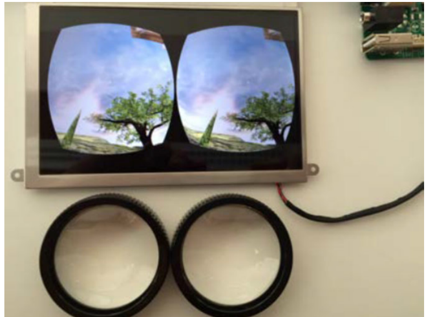
Fig. 4. Prototype screen for the HMD with barrel distortion.
