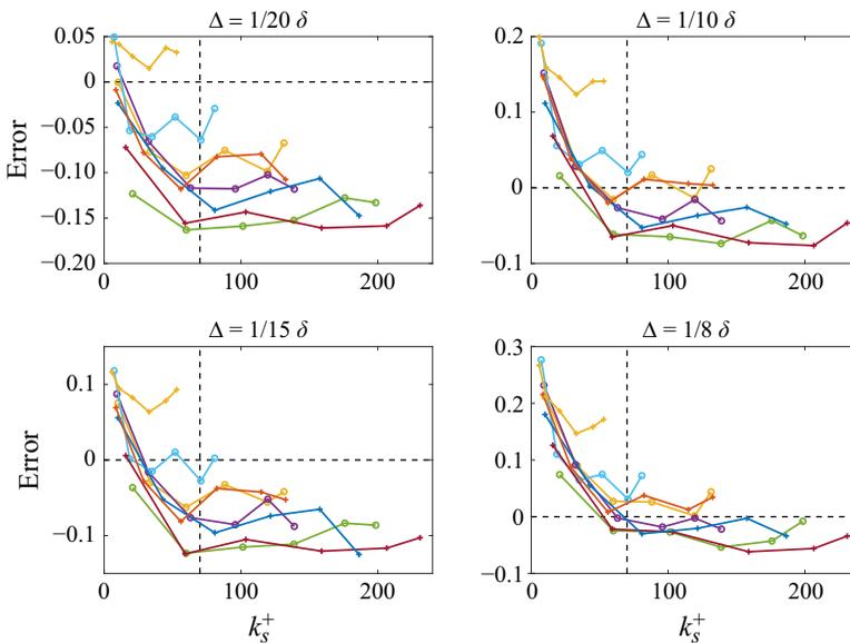
Figure 15. *Aposteriori* error variation of wall-shear stress against  $k_s^+$ . Untrained Weibull and Bimodal rough surfaces are tested in WMLES of turbulent channel flow at  $Re_\tau = 180, 360, 540, 720, 900$  and  $1000$  with trained and untrained grid resolutions, as shown by the symbols with increasing  $k_s^+$ . The error is given as a fraction, and the legend is the same as [figure 14](#).
