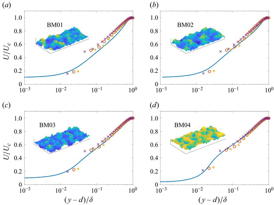
Figure 18. Mean velocity profiles for DNS (line) and WMLES (symbols) of turbulent channel flows at  $Re_\tau = 1000$  with bimodal surfaces: (a) BM01; (b) BM02; (c) BM03; (d) BM04. The roughness geometries are visualized with a section of  $\delta$  in  $x$  and  $0.5\delta$  in  $z$ . Three grid resolutions are visualized:  $\Delta/\delta = 1/20$  ( $\circ$ );  $\Delta/\delta = 1/15$  ( $+$ );  $\Delta/\delta = 1/30$  ( $\times$ ).
