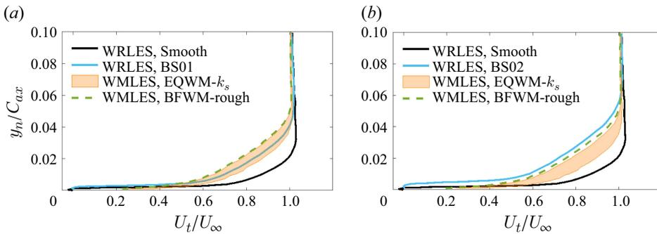
Figure 23. Mean tangential velocity at  $x/C_{ax} = 0.99$  normalized by the local freestream velocity  $U_t/U_\infty$  along the blade-normal direction normalized by axial chord length  $y_n/C_{ax}$ . (a) Roughness BS01 and (b) roughness BS02. The WRLES results of smooth and rough surfaces are from Jelly *et al.* (2023). The shaded area denotes the WMLES with EQWM- $k_s$ , where  $k_s = \alpha k_{rms}$ , and  $\alpha = 3 \sim 7$ .
