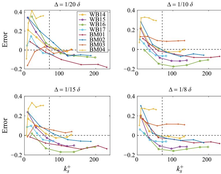
Figure 14. *Apriori* error variation of wall-shear stress against  $k_s^+$ . Untrained Weibull and Bimodal rough surfaces are tested for  $Re_\tau = 180, 360, 540, 720, 900$  and  $1000$  with trained and untrained grid resolutions, as shown by the symbols with increasing  $k_s^+$ . The error is given as a fraction. Note that these selected untrained rough surfaces are the most challenging test cases with the least confidence scores.
