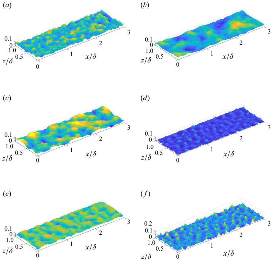
Figure 1. Visualization of roughness height for selected surface samples: (a–c) Gaussian roughness; (d–f) Weibull roughness. The colours represent the level of  $k/\delta$  from 0.0 (blue) to 0.12 (yellow), where  $\delta$  is the channel half-height.
