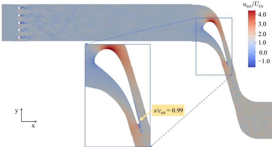
Figure 21. Visualization of the instantaneous axial velocity field normalized by the axial mean inlet velocity  $u_{ax}/U_{in}$  for WMLES of the HPT blade. The arrow indicates the location at 99 % of the axial chord length for probing the mean tangential velocity.
