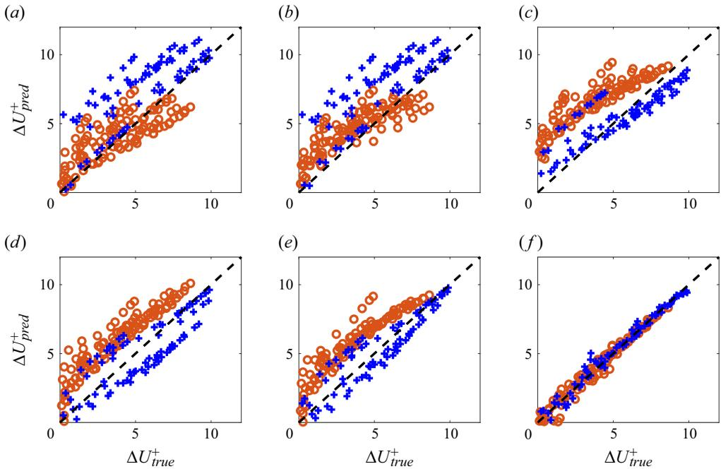
Figure 11. Comparison with rough-wall models from table 7 on the overall 192 rough cases in § 3.4: (a) model for  $k_s^+$  from Flack *et al.* (2020); (b) model for  $k_s^+$  from Kuwata & Kawaguchi (2019); (c) model for  $\Delta U^+$  from Chan *et al.* (2015); (d) model for  $\Delta U^+$  from De Marchis *et al.* (2020); (e) model for  $\Delta U^+$  from Bornhof *et al.* (2024); (f) results from the BFWM-rough. Here red circle, Gaussian roughness; blue cross, Weibull roughness.
