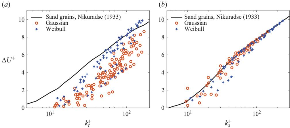
Figure 7. Roughness function  $\Delta U^+$  as a function of (a) mean peak-to-valley roughness height  $k_t^+$  and (b) equivalent sand-grain roughness height  $k_s^+$ . A total of 192 rough cases corresponding to table 4 are included in this plot.
