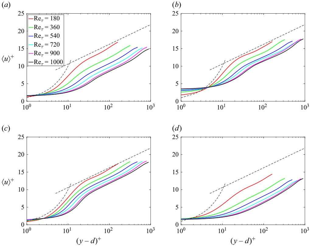
Figure 6. Streamwise mean velocity profiles of selected rough surfaces: (a,b) Gaussian roughness GS01 and GS03; (c,d) Weibull roughness WB08 and WB10. The dashed lines are  $U^+ = y^+$  and  $U_s^+ = \frac{1}{\kappa} \ln y^+ + 5.0$ .
