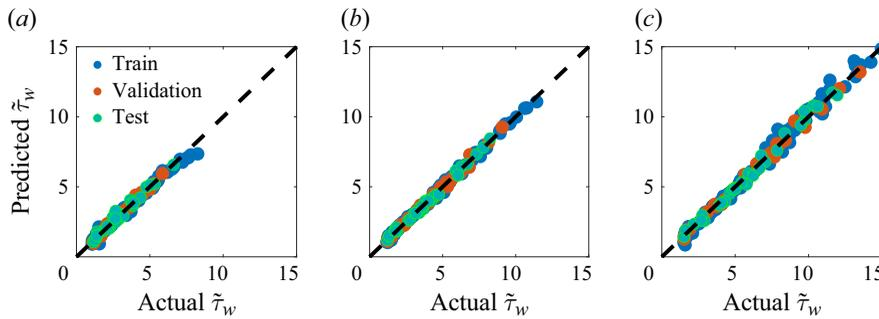
Figure 10. Scatter plot of regression results of actual  $\tilde{\tau}_w$  and predicted  $\tilde{\tau}_w$  for BFWM-rough. The results are plotted for three grid resolutions: (a)  $\Delta/\delta = 1/20$ ; (b)  $\Delta/\delta = 1/10$ ; (c)  $\Delta/\delta = 1/5$ .
