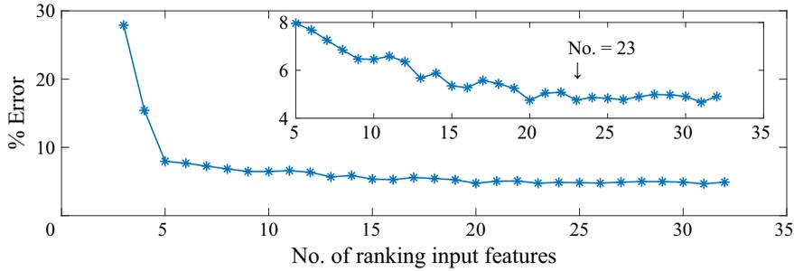
Figure 9. *Apriori*  $L_2$ -norm error in the prediction of  $\tilde{\tau}_w$  as function of the number of input features as ranked in table 5. The inset shows the errors when the number of inputs ranges from 5 to 32.
