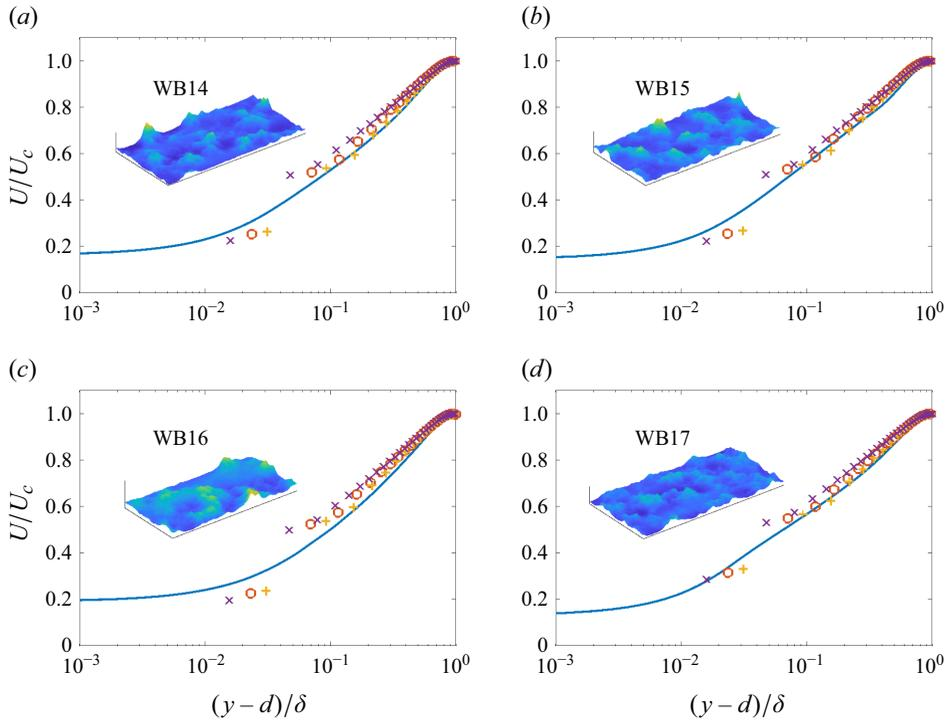
Figure 16. Mean velocity profiles for DNS (line) and WMLES (symbols) of turbulent channel flows at  $Re_\tau = 1000$  with test Weibull surfaces: (a) WB14; (b) WB15; (c) WB16; (d) WB17. The roughness geometries are visualized with a section of  $\delta$  in  $x$  and  $0.5\delta$  in  $z$ . Three grid resolutions are visualized:  $\Delta/\delta = 1/20$  ( $\circ$ );  $\Delta/\delta = 1/15$  ( $+$ );  $\Delta/\delta = 1/30$  ( $\times$ ).
