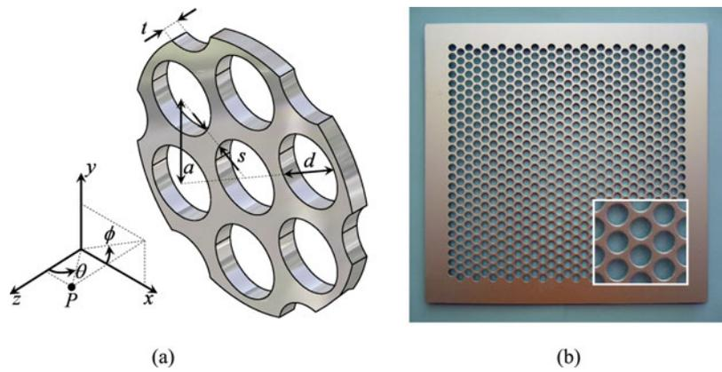
Fig. 3. Prototype of the dichroic mirror: (a) schematic of the unit cell with reference system and (b) photograph.
