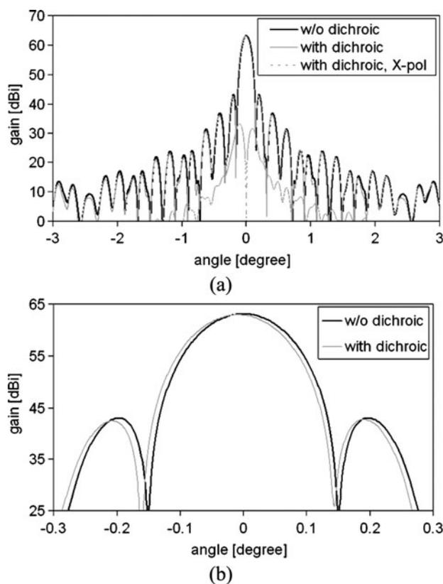
Fig. 5. Simulated 6-m antenna radiation patterns at 26.25 GHz for  $\phi = 45^\circ$ : (a) large-angle view with cross-polarization and (b) narrow-angle view.
