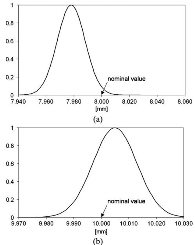
Fig. 6. Statistical distribution of the fabrication accuracy for the test prototype: (a) diameter of the aperture, nominal value 8 mm and (b) separation among apertures, nominal value 10 mm.
