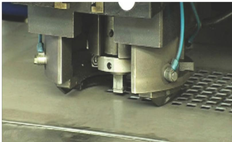
Fig. 2. Example of numerical controlled machine used for punching.
