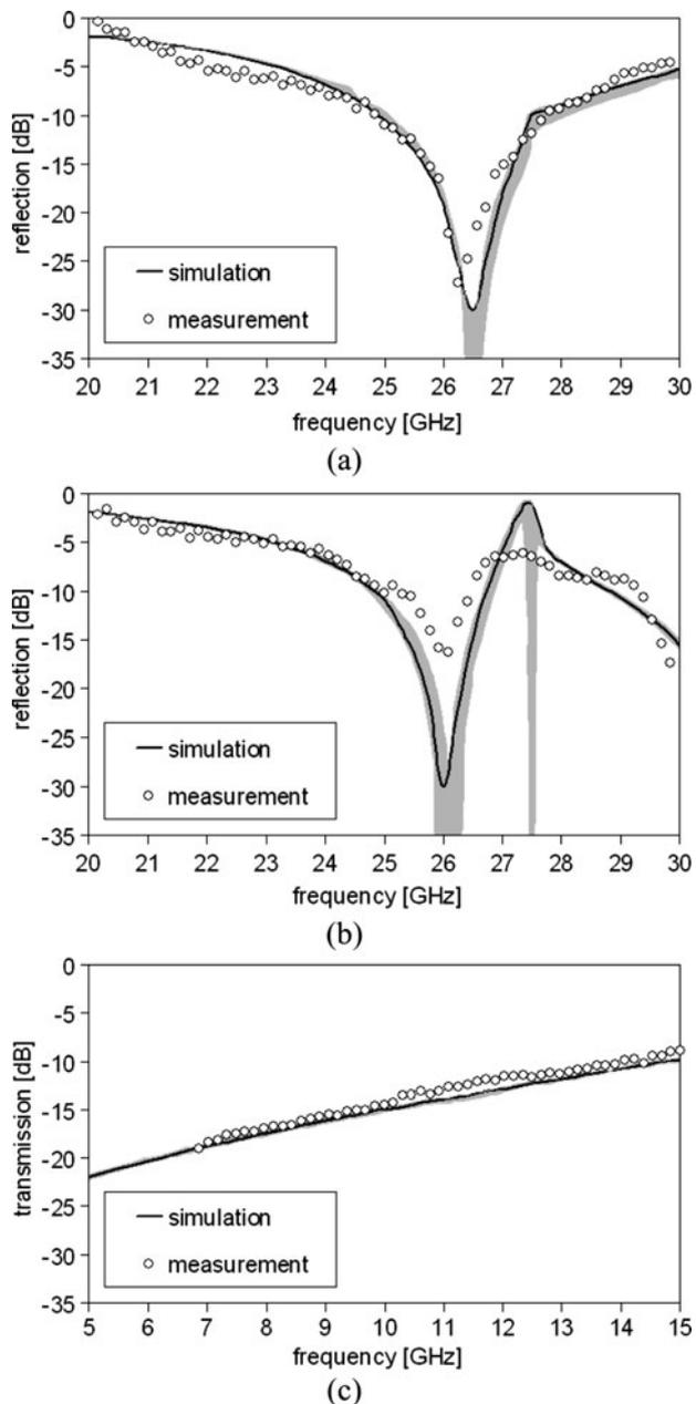
Fig. 7. Simulation (solid line), measurement (circles), and simulated tolerance analyses (light gray bands): (a) TE reflection coefficient in K band; (b) TM reflection coefficient in K band; and (c) TE transmission coefficient in X band.
