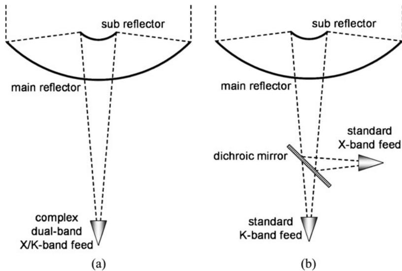
Fig. 1. Schematic of the layout of an antenna working in X and K bands: (a) with single multi-band feed and (b) with two single-band feeds and a dichroic mirror (drawing not to scale).
