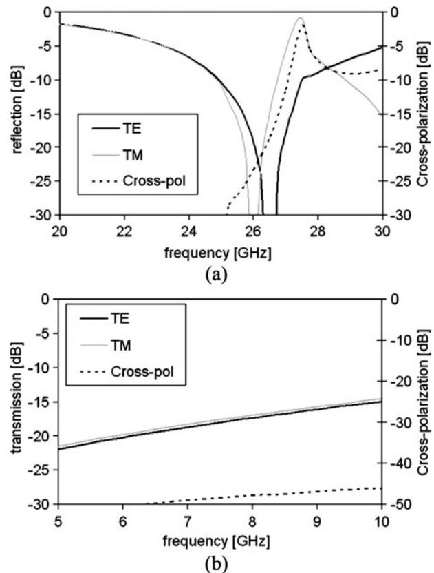
Fig. 4. Simulated performance of the test prototype: (a) reflection for TE and TM modes and cross-polarization for transmitted circular polarization and (b) transmission for TE and TM modes and cross-polarization for reflected circular polarization.
