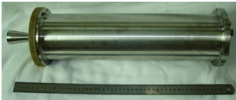
Fig. 30. The photo of coaxial Marx generator.
