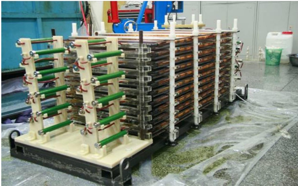
Fig. 26. Photo of pulse generator based on Kapton-film dielectric line.
