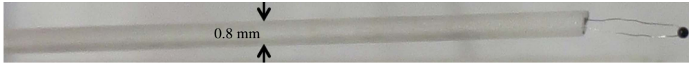
FIGURE 2. Photograph of a Honeywell 111-104HAK-H01 thermistor assembled with its 0.8 mm diameter ceramic rod, ready for insertion into the interior of the cell.
