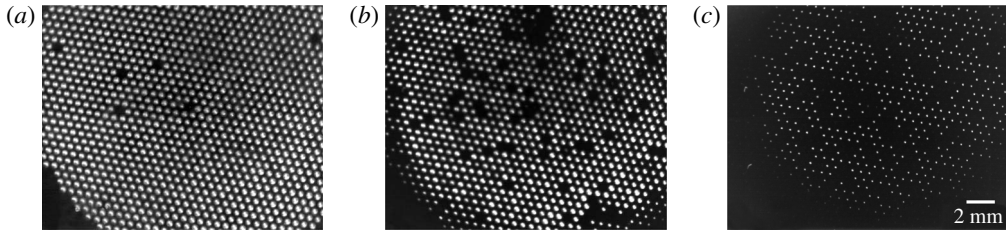
FIGURE 6. Average intensity images of nucleating bubbles on a wafer with cavity spacing l = 0.60 mm at the T_b - T_{on} values given: (a) 9.3 K, (b) 4.7 K, (c) 3.1 K. In (a) all sites except for six (the six dark dots on the lattice) were active. The edge of the etched area can be seen at the left bottom corner. In (b) and (c) an increasing number of sites became inactive.
