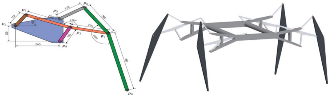
Fig. 4. Standard dimensions of a Klann leg (Left). A 3D model for a quadruped robot using Klann linkages (Right).
