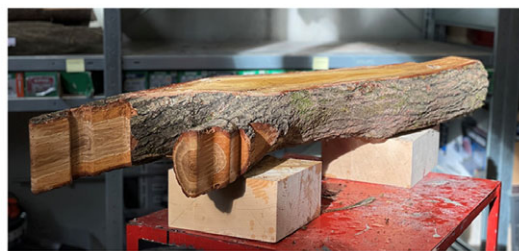
Figure 22. Structural connection: Photo of a construction element from an oak specimen, depicting the position of the contact faces of the joint, considering the central line of the tree's growth.
