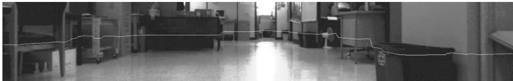
Fig. 11. The curve constructed on the image plane by connecting the laser readings mapped from the laser coordinate frame to image frame.
