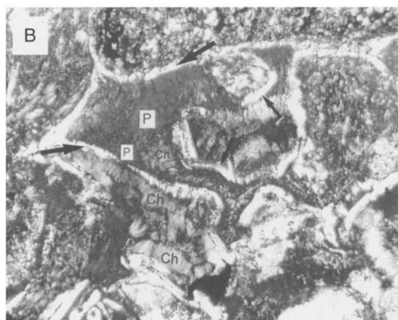
Figure 6. SEM and thin section photomicrographs illustrating textural features of I-S in sandstones. (A) I-S (R = 1) (arrow) coating ankerite crystals (sample DR 24-1, Moranbah Coal Measures, 120 m). (B) I-S pore linings (arrow) covering detrital grains (volcanic-rock fragments) (sample GR 12-10, Moranbah Coal Measures, 519.5 m, field of view = 0.7 mm wide).
