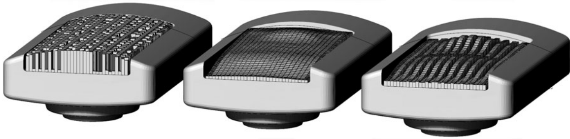
Fig. 8. Examples of the output from three optimization algorithms. Left: maximize thermal dissipation; middle: increase thickness of heatsink in relation to the local temperature; right: user-definable heights in combination with temperature modulation of the remaining geometry.
