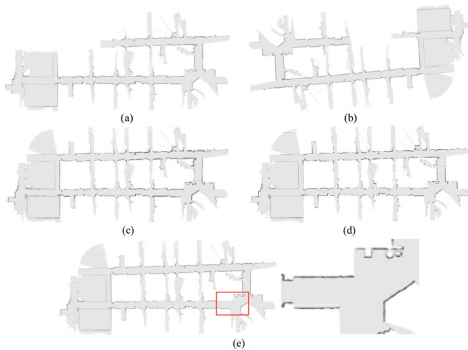
Fig. 11. Merge results of two maps generated from Loop25.log: (a) reference map (5 cm), (b) non-reference map (5 cm), (c) result of Carpin, (d) result of Blanco, and (e) result of the proposed method with enlarged detail.
