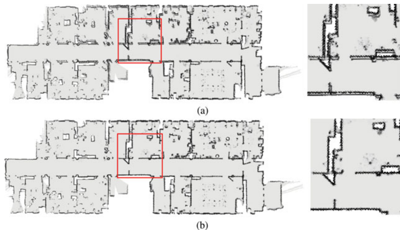
Fig. 6. Map fusion results for different scaling transformations: (a) scaling transformation estimated by all geometrically consistent SIFT matches and (b) scaling transformation obtained by the TsICP algorithm.
