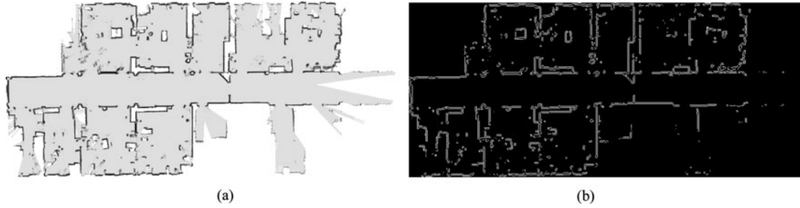
Fig. 1. Edge extraction from a grid map: (a) grid map and (b) extracted edges.
