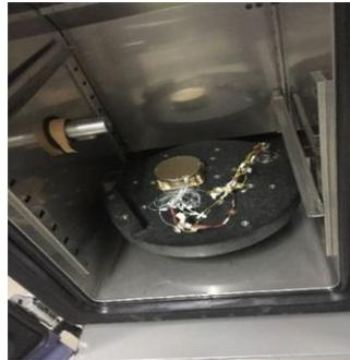
**Figure 7.** Fiber-optic gyroscope calibration experiment.
