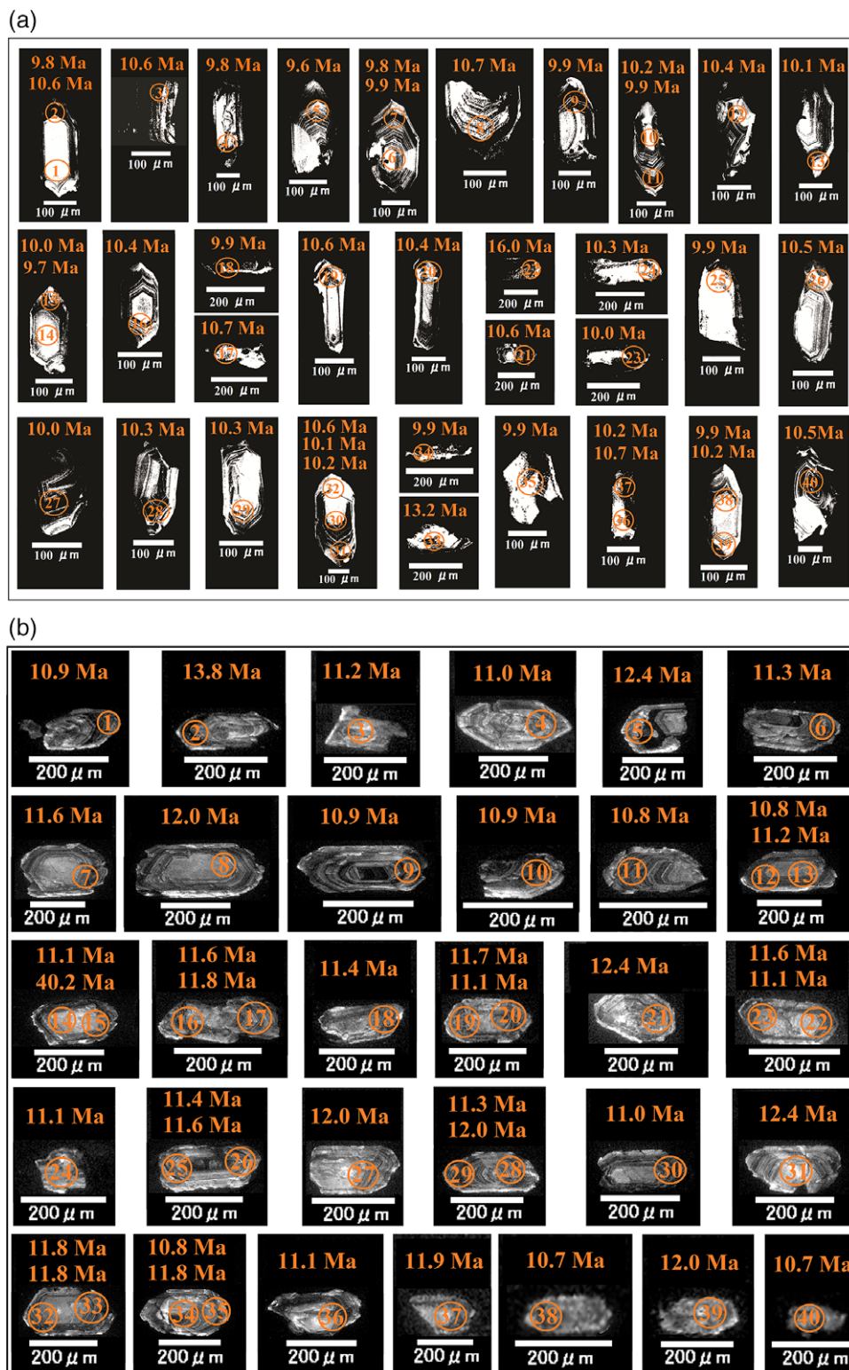
Fig. 6. (Colour online) (a) Cathodoluminescence (CL) images of zircons from sample DKAR11 (rhyolite). (b) CL images from zircons of sample DKAR21 (dacite) with positions of ablation.
