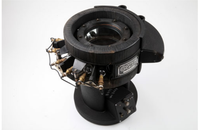
Figure 3. Wilson cloud chamber according to Ballario and produced by Officine Galileo in 1948. The circular illumination surrounding the observation chamber is visible. Copyright © Fondazione Scienza e Tecnica, Florence.
