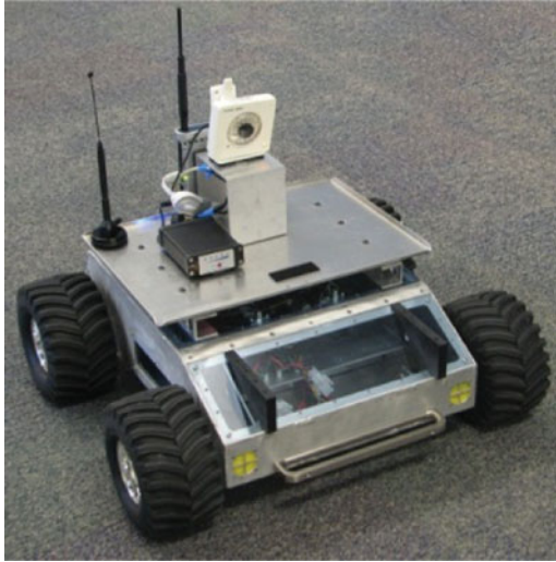
Figure 4. Our Superdroid ATR skid-steer robot instrumented for tele-operation.
