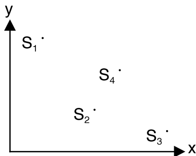
Fig. 8. An example of what Pareto optimality means. If our goal is to find a solution that minimizes both x and y , then S_1 , S_2 , and S_3 are Pareto optimal but S_4 is not.
