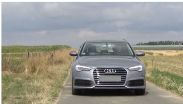
Fig. 6. Station wagon used as cooperative moving radar target driving along a country road with speeds of 50 km/h in one experiment and more than 100 km/h in a second experiment.
