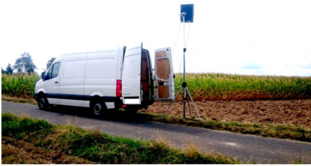
Fig. 5. Installation of the X-band noise radar demonstrator (50 MHz bandwidth, ERP <2 W) in the field with two staring horn antennas mounted at a height of 3.5 m looking along a country road.
