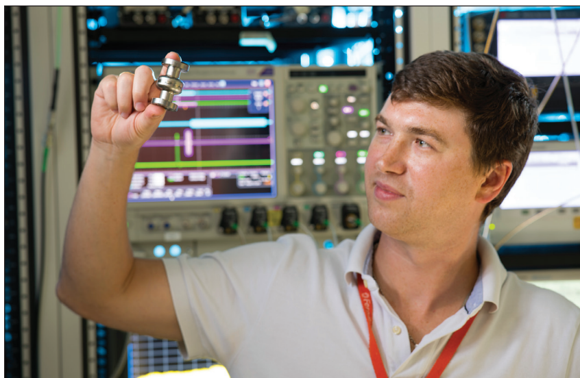
Scientist Alex Romanenko holds up a small superconducting radio-frequency (SRF) cavity in Fermilab’s Quantum Laboratory. Fermilab specializes in SRF cavities for particle physics and is now extending their applications into the world of quantum science. Credit: Reidar Hahn, Fermilab.
