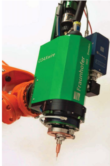
Fig. 6. COAXwire laser head mounted on KR30 KUKA Robot (courtesy of Fraunhofer IWS).
