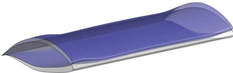
Figure 14. (Colour online) Swept wing redesign case between two symmetry planes with twist, thickness and camber change. Designed wing surface is given in dark colour shade and target wing geometry (untwisted) in light colour shade.
