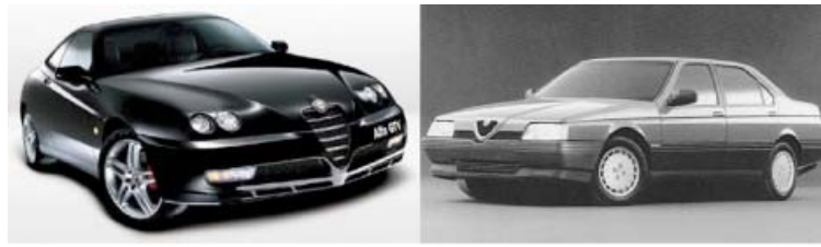
Fig. 1. An example of brand identity pattern: the front hood character lines and grill of Alfa Romeo cars (GTV and 164). Photos courtesy of Alfa Romeo and Pininfarina.
