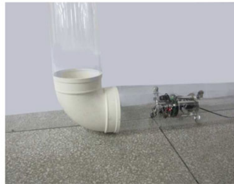
(b) moving inside a pipe
