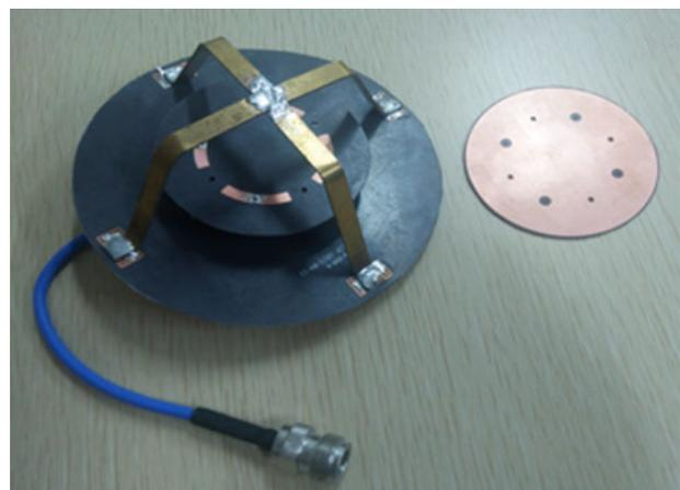
Fig. 5. Photograph of fabricated antenna and top substrate.
