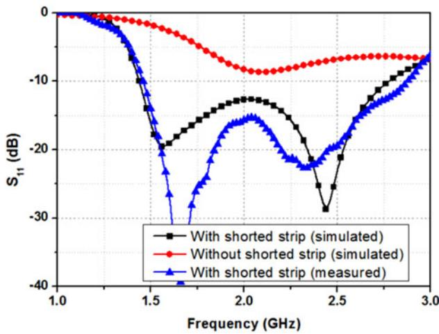
Fig. 2. Simulated and measured reflection coefficients of proposed antenna at different cases.
