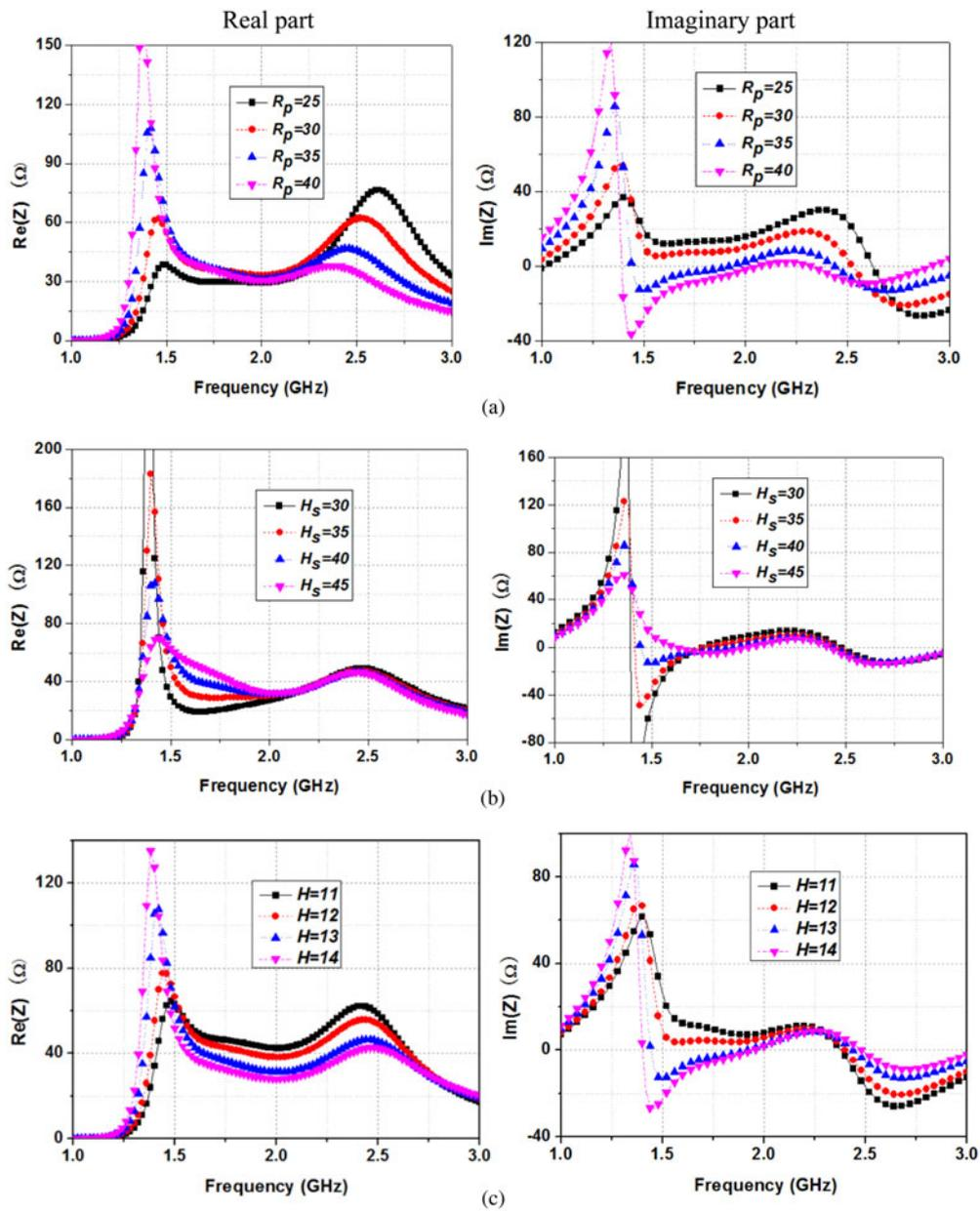
Fig. 4. Simulated input impedance  $Z$  versus frequency with different values of structural parameters. (a)  $R_p$ , (b)  $H_s$ , (c)  $H$ .
