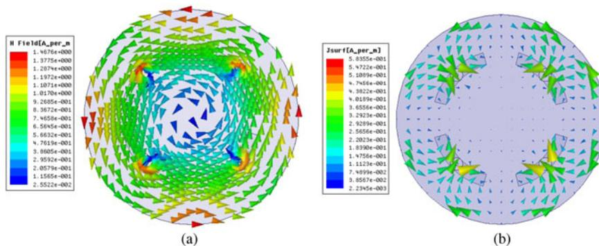
Fig. 3. Magnetic fields and surface current distribution on the circular patch. (a) Magnetic fields, (b) surface current.
