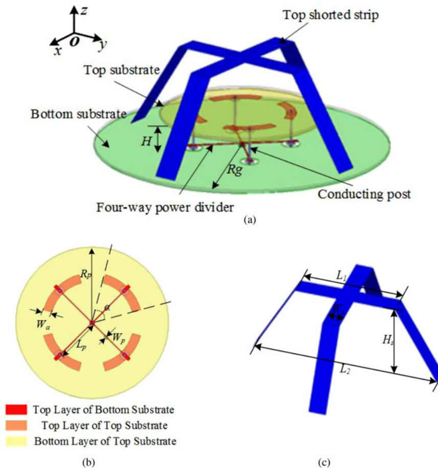
Fig. 1. Geometry of the proposed antenna: (a) over view, (b) bottom view of power divider and top substrate, (c) cross-connected shorted conducting strip.
