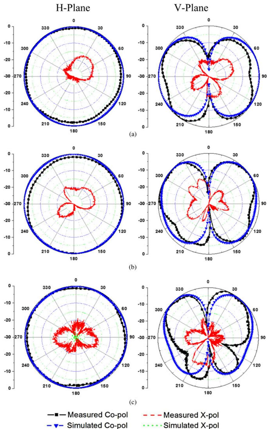
Fig. 6. Simulated and measured radiation patterns of proposed antenna at different frequencies. (a) 1.5 GHz, (b) 2.0 GHz, (c) 2.5 GHz.
