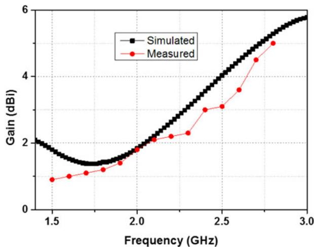
Fig. 7. Comparison of simulated and measured gains of proposed antenna.
