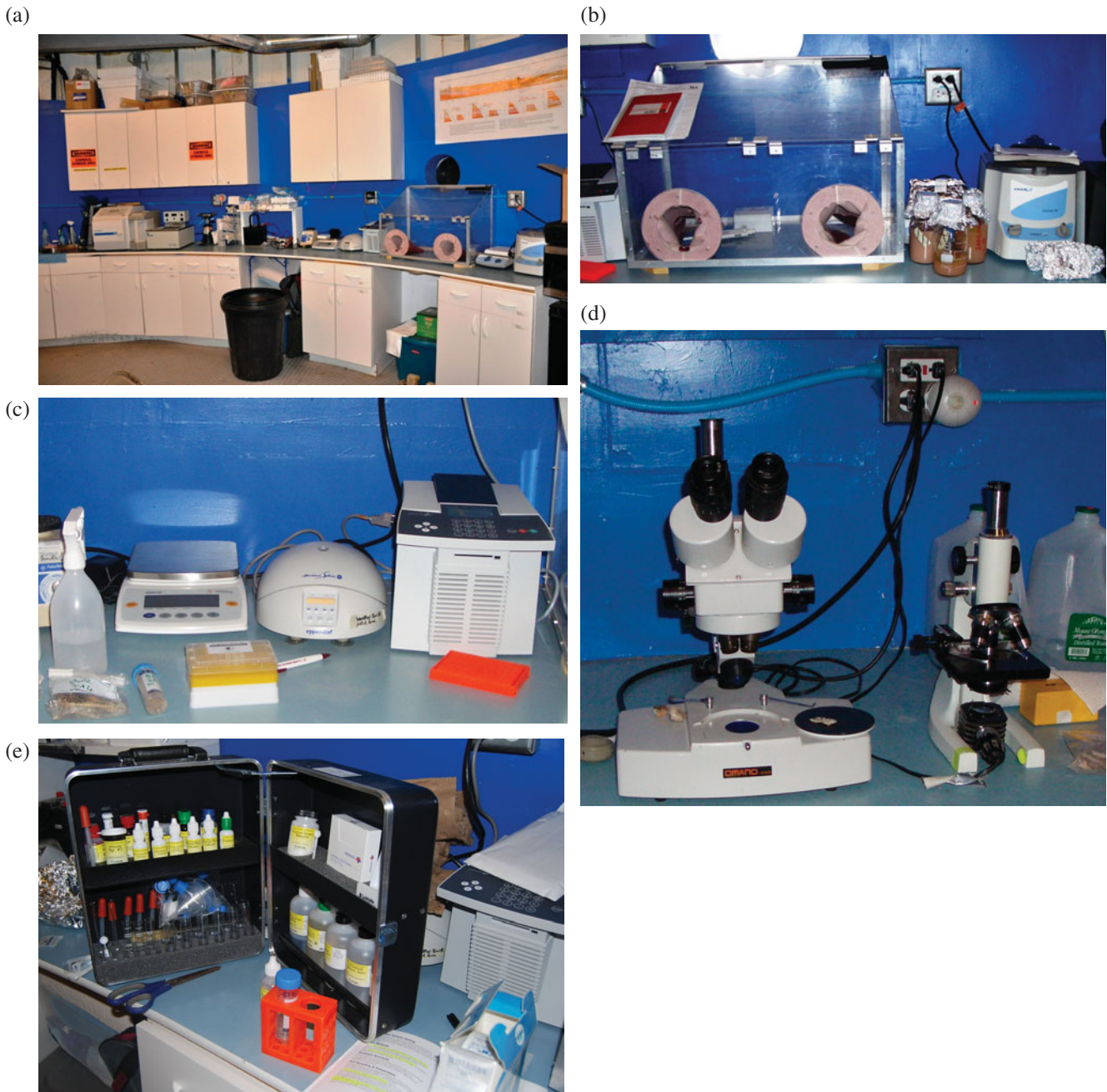
Fig. 9. (a) Installed biology and astrobiology laboratory. (b) Glovebox and sample handling. (c) Precision balance, centrifuge and PCR Peqlab. (d) MDRS microscopes. (e) Soil analysis kit.
