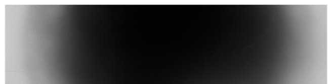
Fig. 8. Darkening of RF-2 film with size 23 \times 86 mm placed in an envelope made of black paper of 100 \mu\text{m} in thickness 8 mm distant from 20 \mu\text{m} -Al foil within an impulse. Generator 3. Diode gap is d = 16 mm, cathode number 1.
