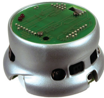
Fig. 6. Description of Khepera-II mobile robot.
