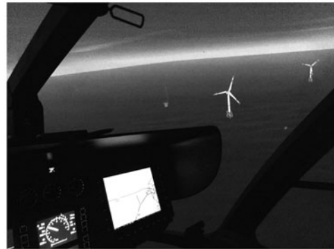
(b) Position of tunnel display in the simulator cockpit.
