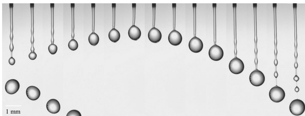
FIGURE 1. The ‘gobbling’ phenomenon: a large terminal drop periodically develops at the end of a thin jet of a viscoelastic fluid (100 ppm PAA solution, Q = 39.7 \text{ mm}^3 \text{ s}^{-1} , R_i = 0.125 \text{ mm} ). A sequence of video images is shown; the time interval between consecutive images is 6 ms.
