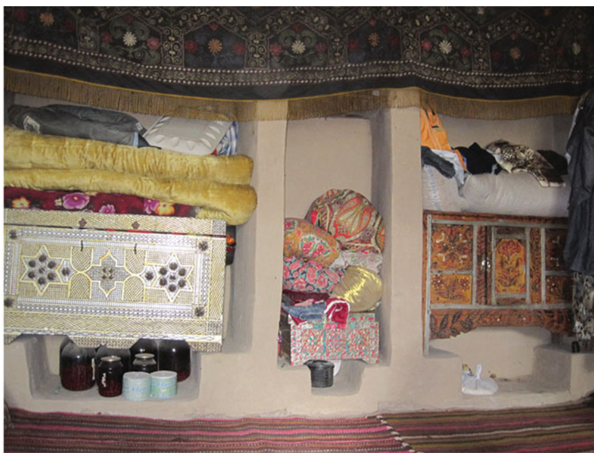
Figure 1. Potential combustibles within traditional houses. Niches within a traditional mud-brick house in present-day Uzbekistan filled with wooden boxes, bedding and textiles, while wool carpets cover the floors.
