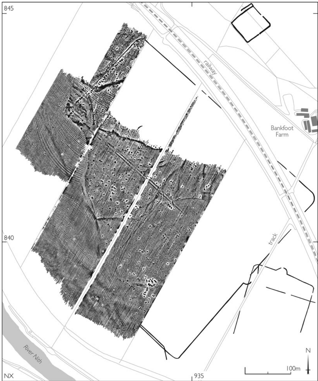
FIG. 7. Grey-scale graphic of the magnetic survey by SENSYS at Bankfoot superimposed over the aerial photographic plot of the camps and postulated two-phase fort. Black-white palette: \pm 3nT . (© Copyright and database right 2018 Ordnance Survey licence number 100057073)
