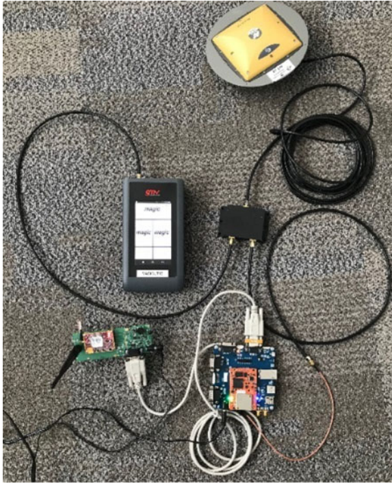
Figure 4. MagicUT and Piksi Multi hardware setup.
