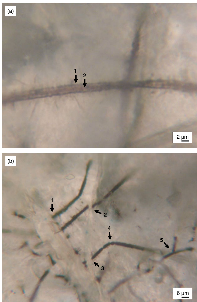
Fig. 5. (a) A photomicrograph in plane-polarized light of a sheeted filament. Two arrows pointing to (1) the outer layer and (2) the inner layer. (b) A photomicrograph in plane-polarized light of filaments that are cut off by the fracture-filling hydrothermal alteration minerals (arrows 1–3). Note also segmentation (arrow 4) and branching (arrow 5).
